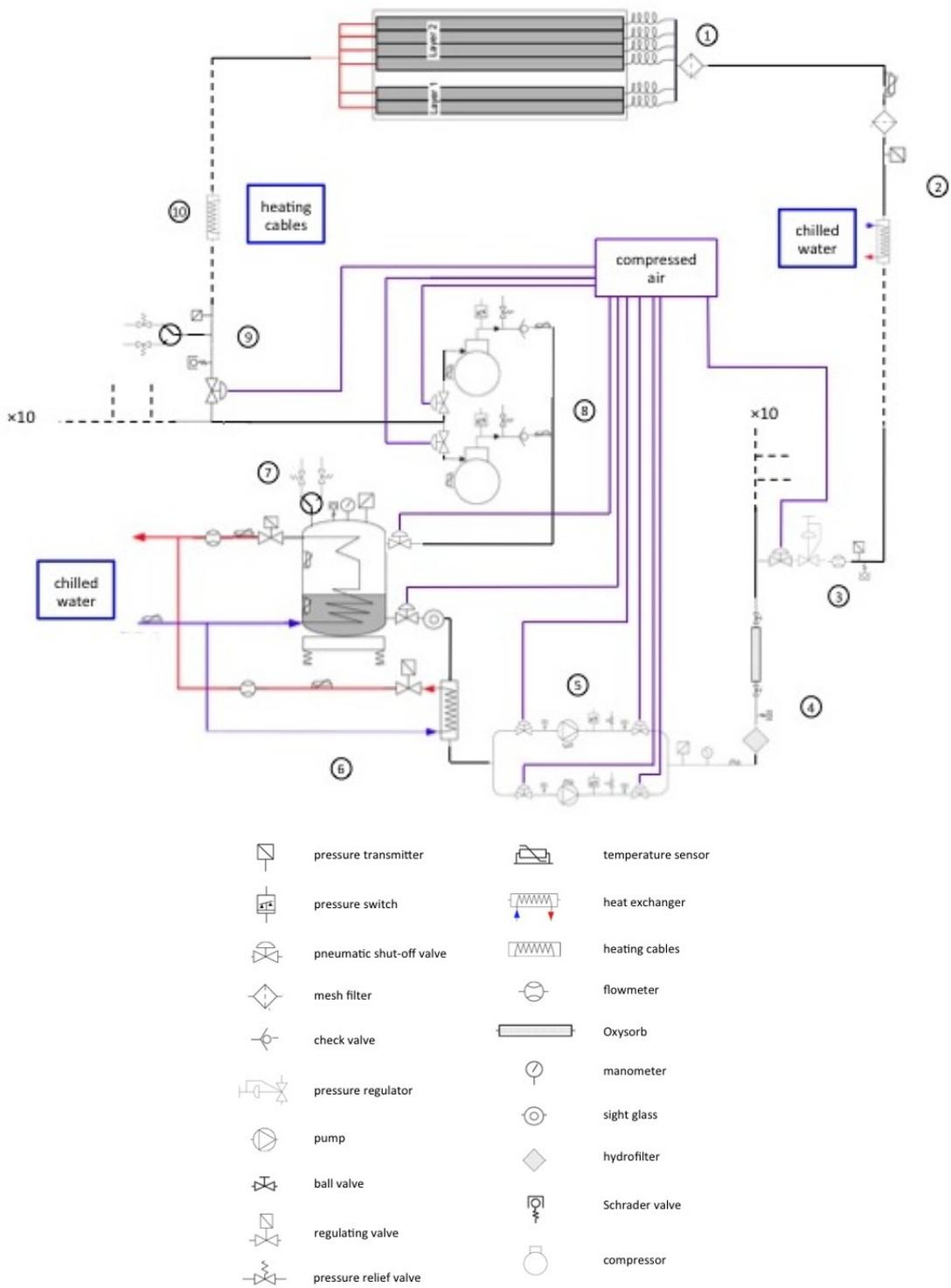
Figure 1: Layout of the SPD cooling circuit.
