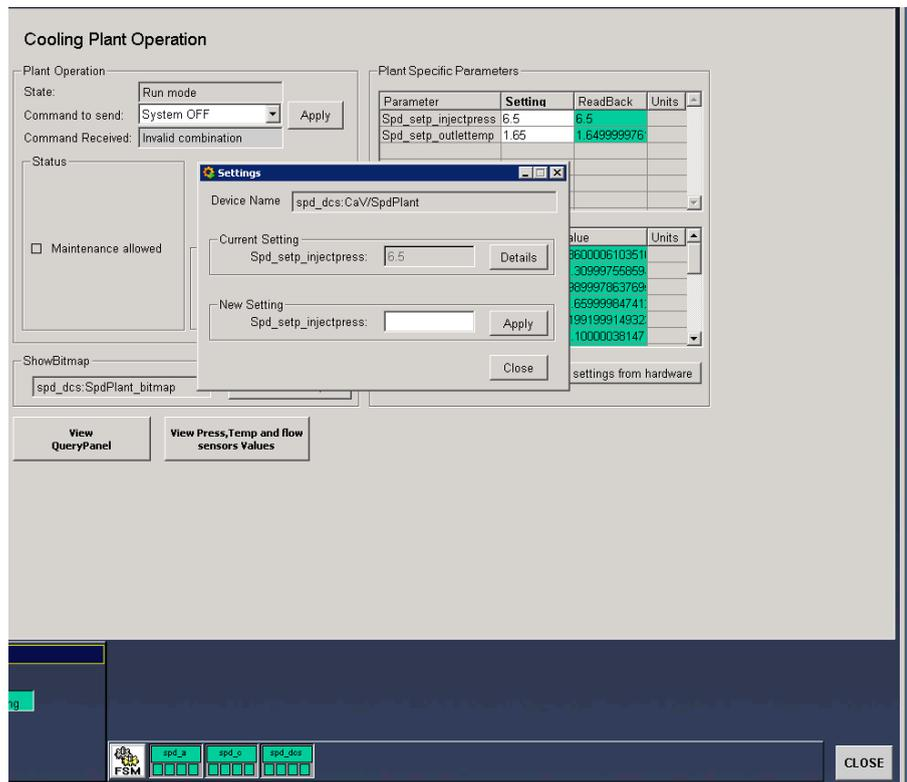
Figure 7: The pressure set panel which pops up when you clic on the value (white field) in the main panel (see text).
