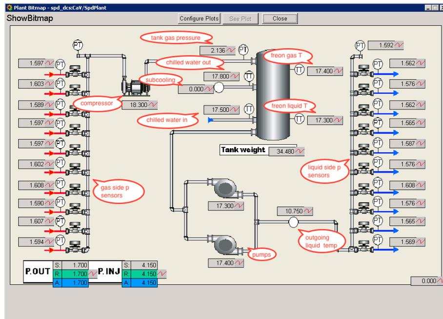
Figure 8: System monitor panel.
