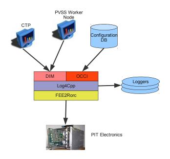
**DIM**: Developed at CERN stands for Distributed Information Management System. It provides a network transparent inter-process communication layer. It is used by the SPD FED to publish status information and to receive commands from other computers through the network.
